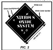
The mark will be clearly visible and will be located in a place which is not likely to be damaged in the event of an accident and which is near to the competition number. Venting and refilling of N2O bottles should be undertaken with extreme caution. External heating of bottle(s) by electric blanket for the purpose permitted.
