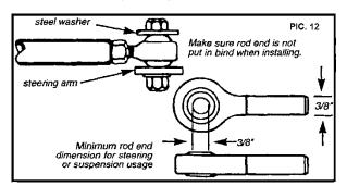
Hollow rod ends are prohibited. All steering boxes, sectors and shafts must be mounted to the frame or suitable crossmember and cannot be mounted in any case to the bellhousing and/or bellhousing adapter shield, motor plate or firewall. Commercially available quick-disconnect steering wheels permitted (except as noted in Class Requirements). All fasteners should be Hex Grade 5 or better, clearly identifiable. No set screws.
