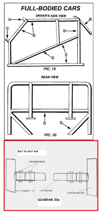
All cars with an O.E.M. frame must have roll cage welded to frame.
